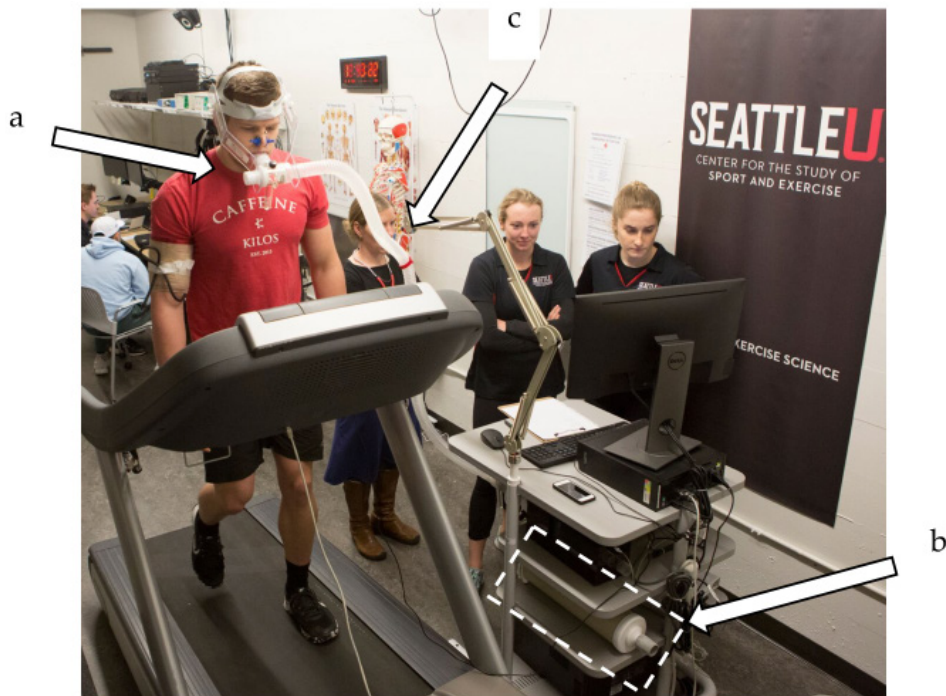
Figure 1 Parvomedics TrueOne 2400 integrated metabolic measurement system. Test subject running on a treadmill, 2017, wearing the snorkel like mask (a) which connects to the mixing chamber on a cart (b) via the connecting hose (c).
